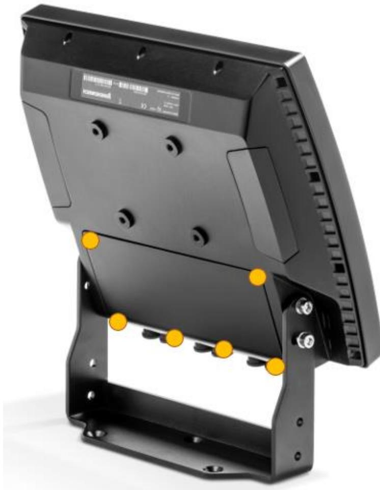
Remove the screws from the service chamber cover (Fig. II, item 4) using a Torx Tx10 screwdriver. Remove the service chamber cover from the terminal.
