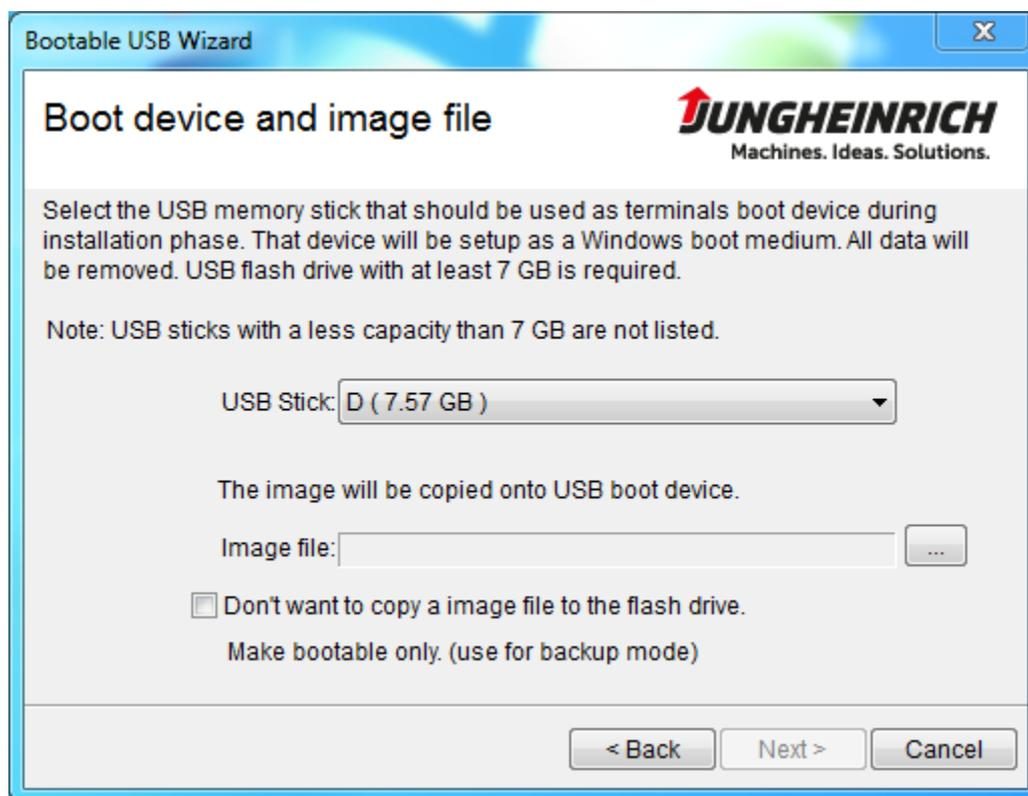
Continue with “Next” and check the settings before you finish the process with “Finish”. The USB stick is then formatted and prepared for installation
