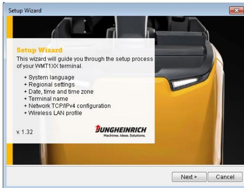
The Jungheinrich WMT Setup-Wizard can be used to set up the WMT and starts automatically at the first boot. The „WMT Setup Wizard” can set up the following configurations.
